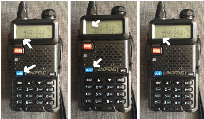
(a) Initial Position (b) A/B Pressed (c) Toggled Again
